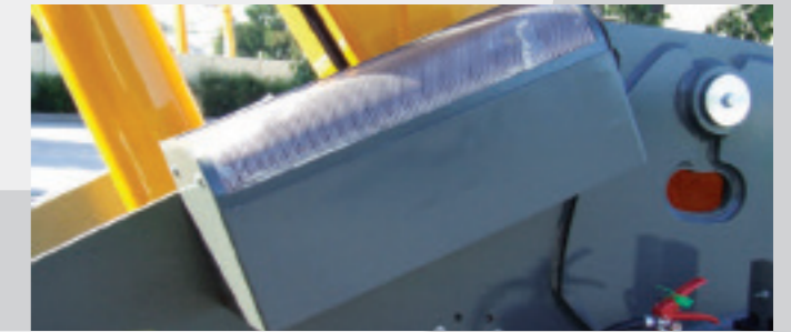
Independent hydraulic coil cooler relocated behind cab with twin auto reversing cooling fans
