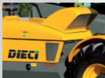
Clean air intake bonnet with fine mesh
