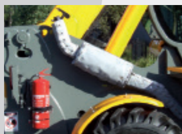
Turbobank heat protection from turbo to end of exhaust pipe
