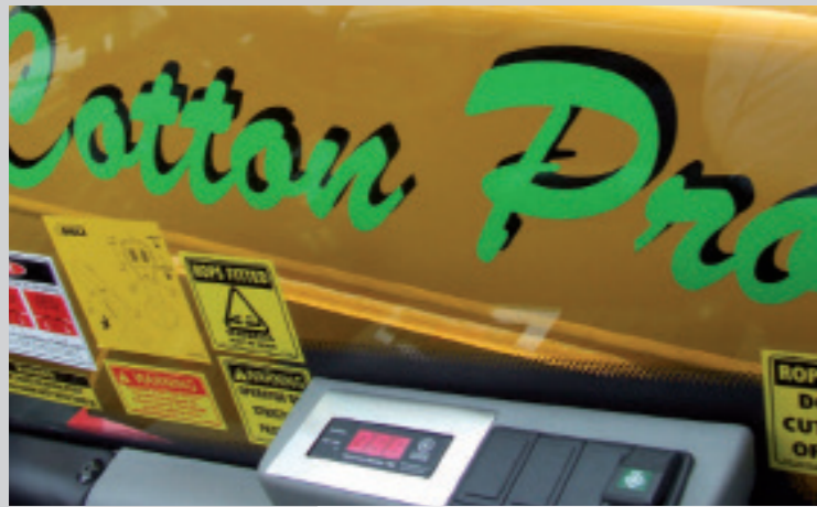
Engine temperature monitoring system with shutdown protection
