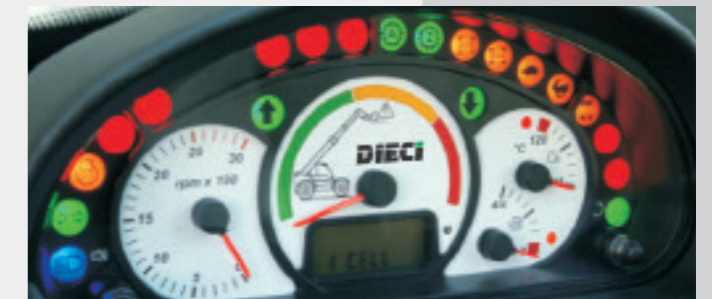
Modern integrated instrument panel with load management readout
