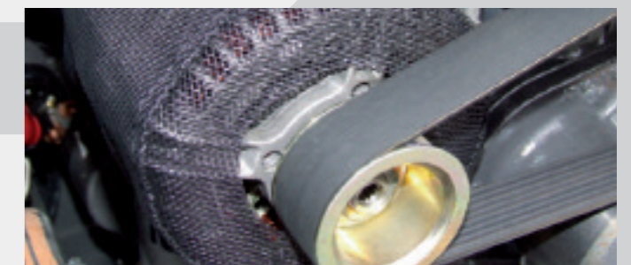
12V system 2 stage 90amp alternator with fibre sock cover for protection
