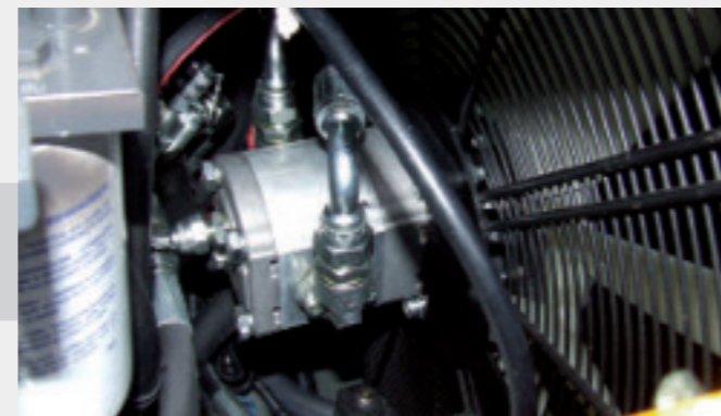
Hydraulic reversing fan on engine radiator
