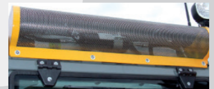
Air conditioning with automatic reversing condenser fan every 20 mins along with protective cover and stainless steel mesh
